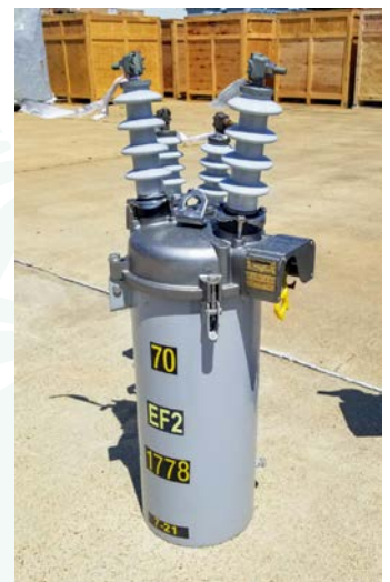
Oil Circuit Recloser sitting on the ground
